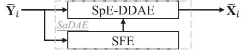
Figure 2: The block diagram of the proposed SaDAE, which includes the SpE-DDAE and SFE components. The system input is the frame-wise noisy feature vector \tilde{\mathbf{Y}}_i , while the output is the enhanced feature vector \tilde{\mathbf{X}}_i .
